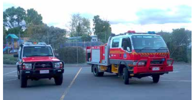
Taroona 5.1 and Taroona 4.1 appliances. Taroona 5.1 is mainly used for bushfire operations. Taroona 4.1 is a dual-purpose appliance. It is equipped with BA gear for structure and vehicle fires, but is also a highly capable bushfire fighting appliance.
